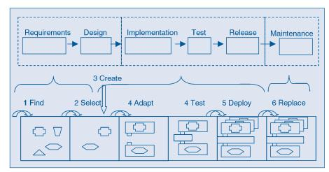
Figure 1 The development cycle compared with the waterfall model
