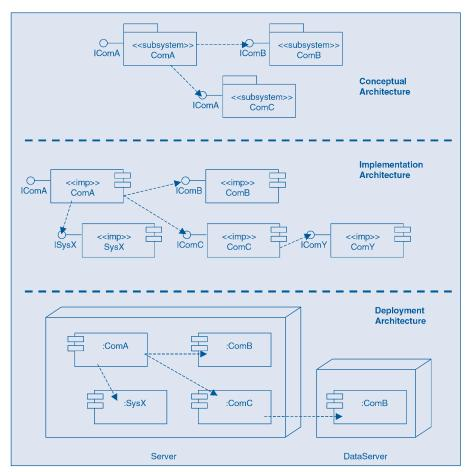
Figure 3 Examples of different aspects of component-based architecture
